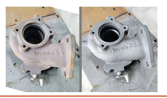
Remote cleaning commonly used for rusty removal and part of coating or painting removal, the cleaning width can reach 80mm
